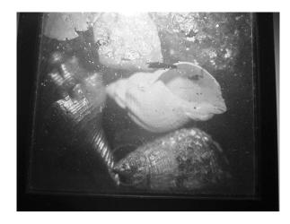
Figure 1. White-Light-Reflection Hologram recorded on DESA silver bromide emulsion (grain size: 15 nm) in Denisyuk single beam geometry with a HeNe-laser (20 mJoules) at 632,8 nm: crystallized rose quartz, pyrit, snail shells
