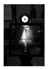
Figure 2. Rain Bow Transmission Hologram recorded on DESA silver bromide emulsion (grain size: 15 nm) in Benton split beam geometry with a HeNe-laser (20 mJoules) at 632,8 nm: faucet
